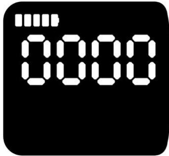
5.7. 3.2 Short time press the add or reduce key to increase or decrease the number, short time press the startup key to jump to the next number setting, and so on:
