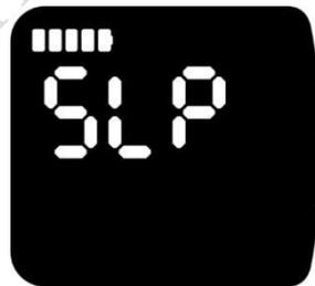
5.7. 5.1 One time press the startup key for a short time, and the display enters the dormant time setting state:
