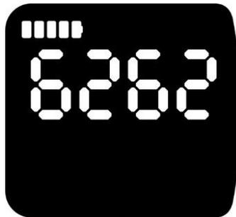
After entering the password "6262", one time press the startup key, and the display enters the next level menu. The display displays "Frt" to restore the factory settings:
