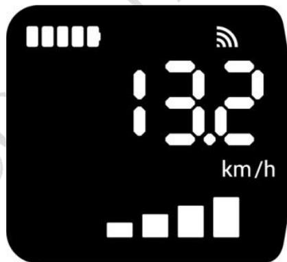
Keep the distance between the mobile phone and the D19 display 10-15m, turn the crank of the whole vehicle, and the interface has corresponding information such as battery power, average speed, etc., indicating that the Bluetooth communication between the D19 display and the mobile phone is normal and the function is normal. Shut down the whole vehicle system, exit the mobile phone APP software, and the test is completed.
