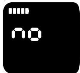
5.7. 3.3. 2 If it is necessary to set the speed limit, in the "LSd" interface, one time press the startup key for a short time. When the display displays "NO", press the add key for a short time to display "20.0" (press the reduce key for a short time to display "70.0"), adjust the speed limit (range 20.0-70.0, and decrease by 0.1 each time), and press the startup key for about 1.5 seconds to confirm and automatically return to the upper level menu.
