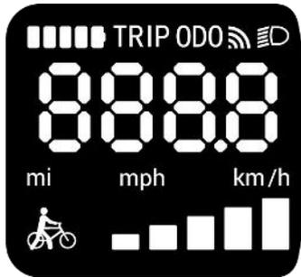
After the whole picture disappears after 1 second, the display enters the working state, displaying the total riding mileage/ODO and real-time speed:
