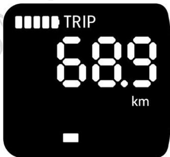
4.2. 2 Short press the startup button again to display the total mileage of a single time/trip time:
