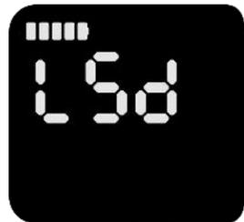
5.7. 3.3. 1 If it is not necessary to set the speed limit, press the startup key once in the "LSd" interface. When the meter displays "NO", press the startup key for about 1.5 seconds to confirm and automatically return to the previous menu.
