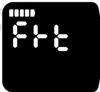
5.7. 3.2. 1 One time press the startup key for a short time, and the display enters the selection state of restoring factory settings, and the display displays "NO". If you don't want to restore factory settings, press the startup key for a long time or press the add or reduce keys at the same time for about 1.5 seconds to return to the upper menu, that is, the "Frt" interface.
