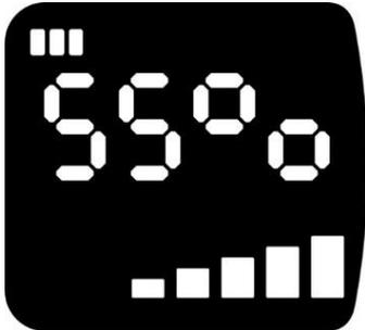
4.2. 4 Short press ON/OFF button to display the riding speed:
